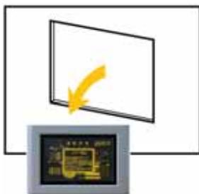
2) Attach panel cut adapter "PAD-V608-1".
