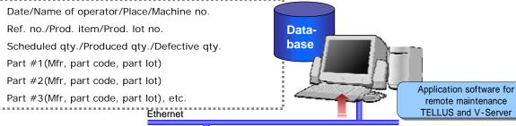
Data such as a 2D code can be read by connecting the barcode reader with V8.
