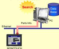
3) Enter the received quantity and write the stock quantity to the database.
