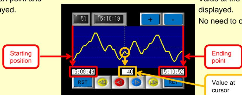
Sampling time display and cursor value is refreshed to update when the cursor moves or display is enlarged.
