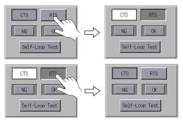
\* Since the V808CH unit does not have [+CTS] and [-CTS] signals for the terminal block TB3 (RS-485 connection), a self-loop test should be performed by using [+RD] (pin 14) and [-RD] (pin 15) signals.
