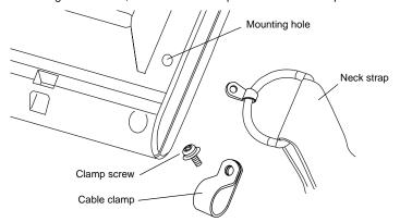
2. Put the cable clamp on the neck strap fixture, and tighten them together using one clamp screw.
