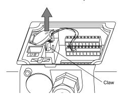
\* Be sure to hold the battery when removing it. Take care not to yank the battery cable.
