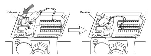
Press the inclined battery downward, and fit the battery under the claws in order to snap it into the battery socket.
