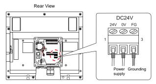
Tighten terminal screws on the power supply terminal block equally to a torque of 0.28 Nem (2.8 kgfecm).
