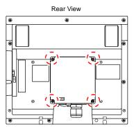
3. Check that the battery is securely attached to the backside of the cover, and connect the battery connector.
